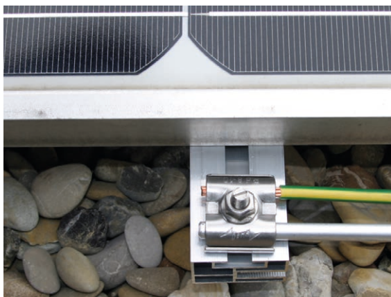
Figure 3 UNI earthing clamp: A stainless steel intermediate element prevents contact corrosion, thus establishing reliable long-term connections between different conductor materials
