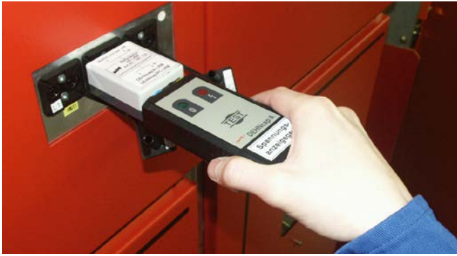
Self-test of a DEHNcap/A voltage indicator.
