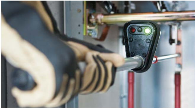
PHE voltage detector with visual indication.
