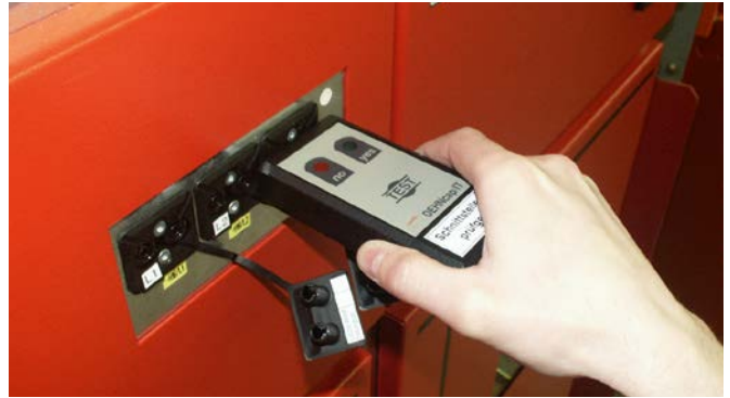
DEHNcap/IT interface test unit allows to carry out maintenance tests on coupling systems of switchgear installations according to IEC/EN 61243-5 (DIN VDE 0682-415).
